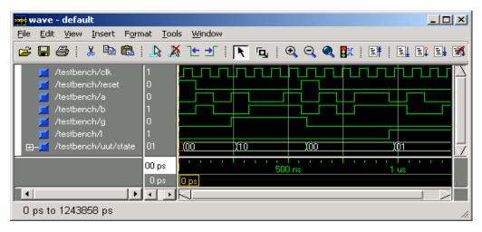
VHDL allows us to define signals with enumerated types so that we can associate meaningful names to values of signals. This is particularly useful for naming the states of state machines, as illustrated below.
