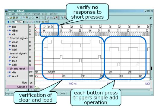
Before we look closely at the actual simulation output, it worth taking a few moments to notice a few things about the waveform display. At the left, where the signal names are listed, the signals have been organized into groups, with labels added to identify each related group of signals.
