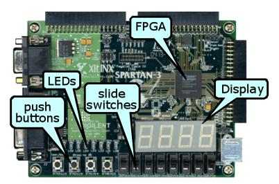
This board contains a Xilinx Spartan-3 FPGA and we'll refer to the board as the S3 board for the remainder of this chapter. In addition to the FPGA, the S3 board has four push buttons and eight slide switches, that can be used to provide inputs to the FPGA circuit, plus eight Light Emitting Diodes (LED) and a four digit numeric display that can be used for
