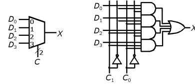
this circuit can be generalized to implement muxes with 8, 16 or more inputs. A *demultiplexor* performs the inverse function of the mux. It has a single data input, k control inputs and  $2^k$  data outputs. If the value represented by the control signals is i, then output  $D_i$  is equal to the data input, while all other data outputs are 0.
