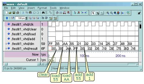
The signal names appear at left, starting with clk, followed by the three control inputs, the data input and the results output. Notice how the clear signal causes the result output to go to zero, how the load signal causes a new value to be loaded from dIn and how the add signal causes the value on dIn to be added to the stored value. Also, note how every change to result happens on the rising clock edge, since this is when the internal register changes.
