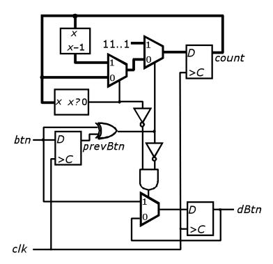
Because the count signal is defined to be 20 bits long, the debouncer will count down for 2<sup>20</sup> clock ticks following a transition on btn, before reflecting that transition at the outputs. Since 2<sup>20</sup> is slightly more than one million and since the period of the clock on the S3 board is 20 ns, this means that the circuit implements a delay of just over 20 ms, which is long enough to filter out any spurious transitions due to vibration of the button mechanism.
