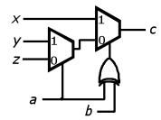
Note the similarity between this and the circuit that implements the ifthen-elsif statement in the calculator circuit from Chapter 2. The conditional signal assignment can have any number of when-else clauses, and each successive clause can be implemented using another multiplexor. We can also use the conditional signal assignments with signal vectors. If A, B and C are all 8 bit signal vectors, then the assignment
