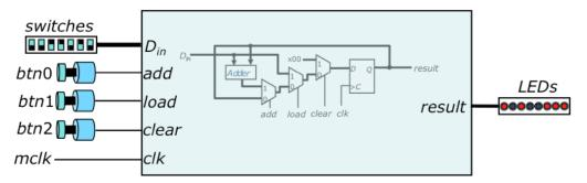
As shown in the picture, we'll connect the slide switches to the data input signal and three of the push buttons to the three control inputs. The external signal mclk is a 50 MHz clock signal that comes from a clock generator circuit on the board and is connected to one of the input pins of the FPGA. We'll connect the calculator's result output to the LEDs on the board.
