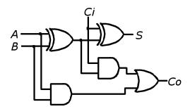
The signal assignments are only one part of a VHDL circuit specification. To completely define a circuit, we must also specify its inputs and outputs. As an example, here is a complete specification of the full adder circuit.
