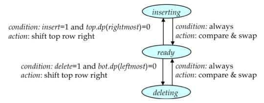
This is a somewhat ideallized state transition diagram, but it captures the essential behavior we want. In particular, the labels on the arrows indicate the condition that causes the given transition to take place and any action that should be performed at the same time. The variable *top(rightmost).dp* refers to the rightmost data present flip flop in the top row and *bot(leftmost).dp* refers to the leftmost data present flip flop in the bottom row.
