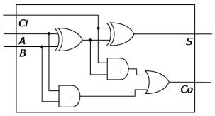
We often find it convenient to define internal signals that are used in other assignments, but are not outputs of the circuit we are specifying. For example, we might specify the full adder using the following assignments.
