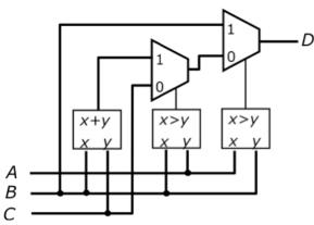
Here the labeled blocks designate combinational sub-circuits that implement an inequality comparison function and an addition function.
