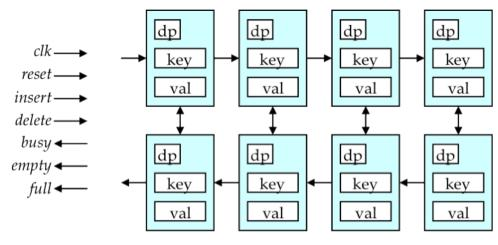
In this design, there is a set of *cells* arranged in two rows. Each cell contains two registers, one storing a *key*, the other storing a *value*. In addition, there is a flip flop called *dp*, which stands for data present. This bit is set for every block that contains a valid (*key,value*) pair. The circuit maintains the set of stored pairs so that three properties are maintained.
